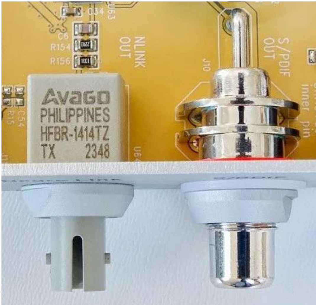
Avago's ultra-fast optical transmitter for N-Link (left), next to the coaxial digital output.
